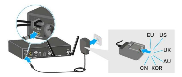
To completely disconnect the EM 100 G4 from the power supply system:
