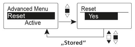
When you reset the wireless microphone, only the selected settings of the pilot tone and the  ${\bf U}$  frequency bank are retained.
