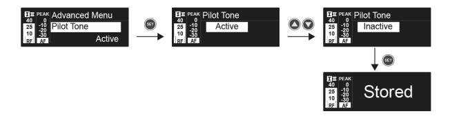
The pilot tone has an inaudible frequency that is sent from the transmitter and evaluated by the receiver. It supports the receiver's squelch function.
