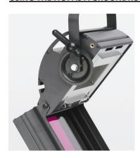
The **HUI** can also be used as a groundrow. To modify the **HUI** for groundrow operation, reverse the colour cassette assembly by removing the two screw pivot hinges located on each side of the luminaire. Invert the colour cassette, then replace the two screws in the new hinge position.
