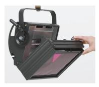
To remove the colour frame, open the hinged door at the top of the colour cassette and lift out the frame. Use the colour frame as a template to cut a colour filter to the exact size of 264mm x 202mm.
