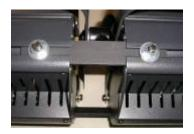
Single HUI units can be joined together to make multi unit battens. To join units together, position the yokes in the vertical position, and lock off. Place the Hui units side by side and slide the slot lock bars (Order Code 15HLI) into the top and bottom join slots. Tighten the slot lock nuts with a wrench. Repeat until the desired number of units are joined.
